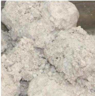
**Purified phosphogypsum** still contained toxic heavy metals above the levels demanded by plasterboard manufacturers
