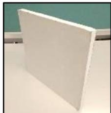
**ICEBERG plasterboard prototype with 35% purified gypsum from EoL plasterboard fulfills the mechanical and thermal requirements for standard plasterboards.**
