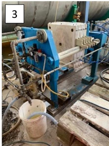
Step 1 - Acid leaching purification of gypsum from End-of-Life (EoL) plasterboard at 90°C for 1 hour using a 5 wt% sulfuric acid solution.
