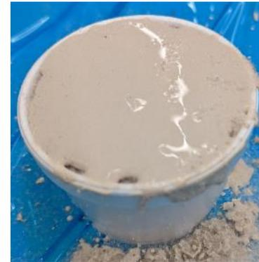
**SICLA aerogel** and gypsum cannot create the required homogeneous blend for plasterboard production
