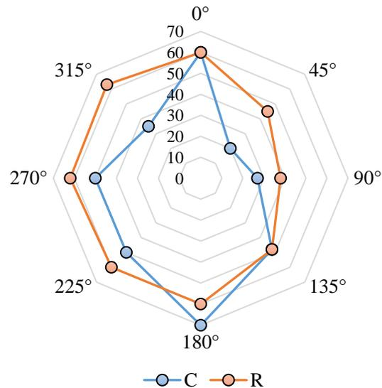
Figure 47. Average readability of 'CS' RFID tags in cm in concrete beam (C-centre and R-right)
