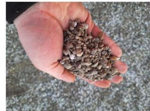
Figure 35. Recycled crushed 4/10
