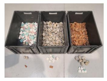
Average Particle Weight: 36.5 g (Concrete); 22.4g (brick); 25.5 (gypsum)
