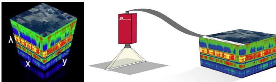
Figure 7. Conceptual scheme of a hyperspectral image (two spatial and one spectral dimensions)
