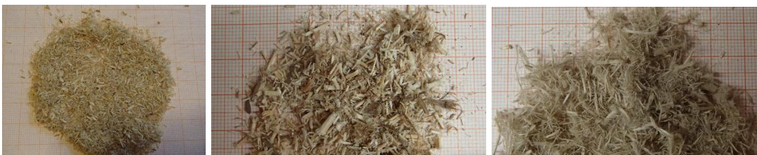
Figure 55. Pure C&D wood fractions after processing with hammer mill (left), Pallmann PSKM (middle) and disc refiner (right).
