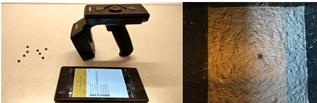
Figure 18. The RFID reader and writer system (left). RFID embedded in concrete (right).
