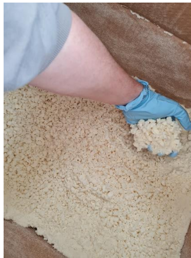
Figure 79. Example for the PUR/PIR insulation boards after grinding for usage, like lab-scale experiments.
