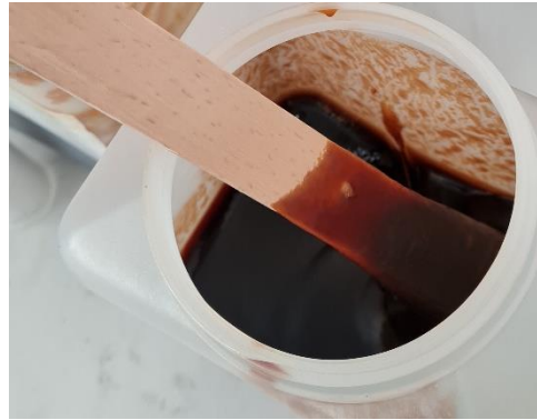
Figure 81. Example of a finished polyol from degraded PUR insulation boards.
