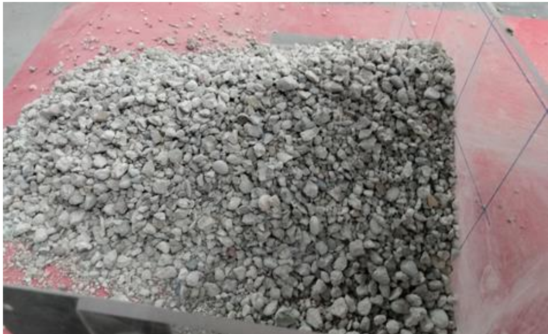
Figure 25. Side view of the heap profile for coarse fraction aggregates.
