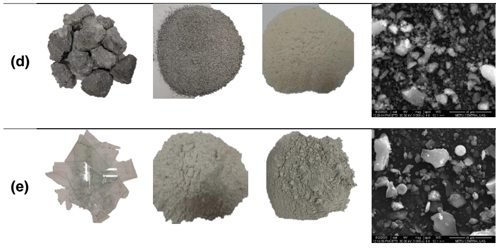
Figure 2. Photographs and SEM Images of CDW-based materials: (a) Red Clay Brick, (b) Hollow Brick, (c) Roof Tile, (d) Concrete Waste, (e) Glass Waste
