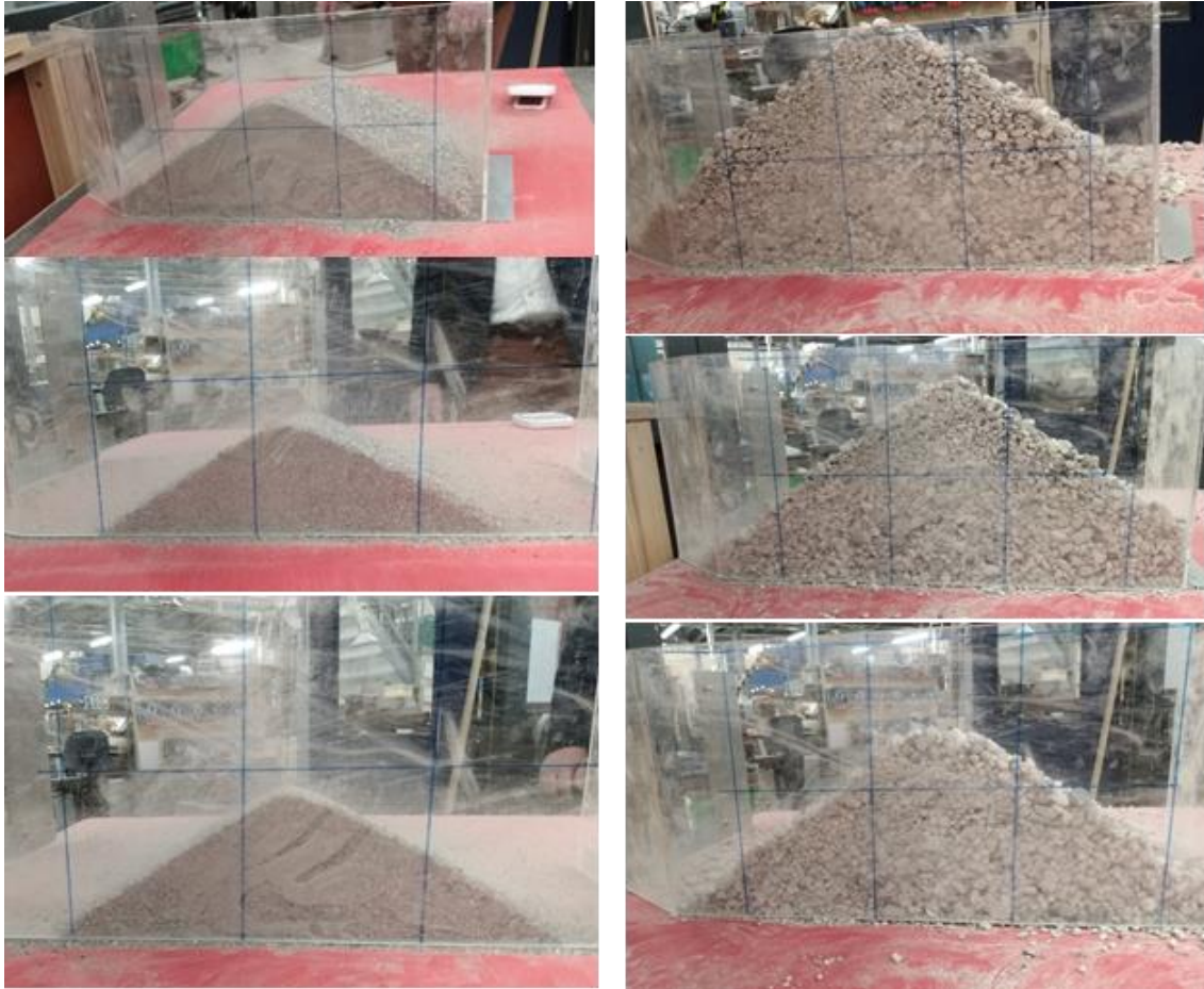
Figure 24. The heap shape for aggregates of different size (Left: Fine fraction and Right: coarse fraction).
