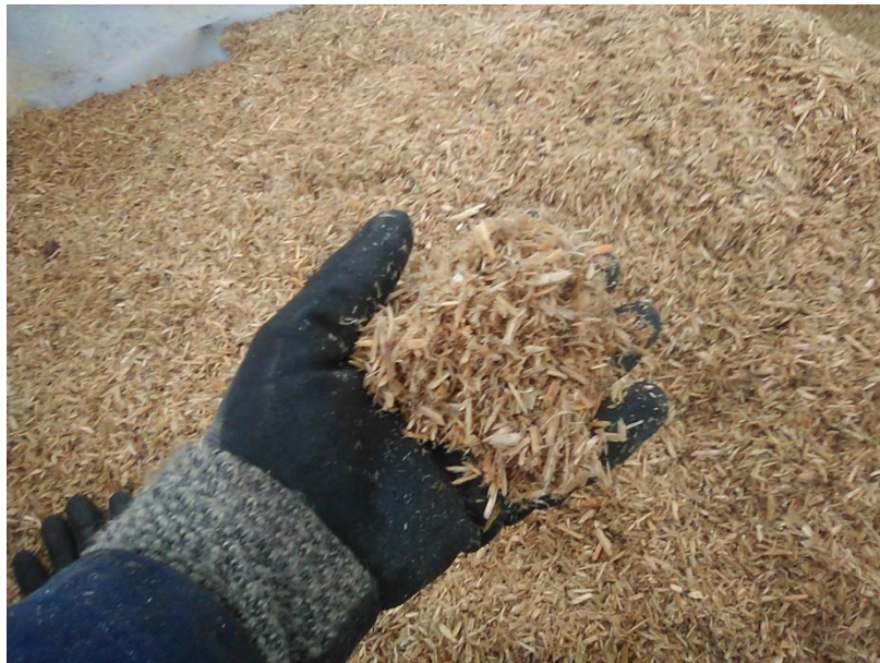
Figure 54. C&D clean wood fraction after processing with hammermill equipped with 8 mm sieve.
