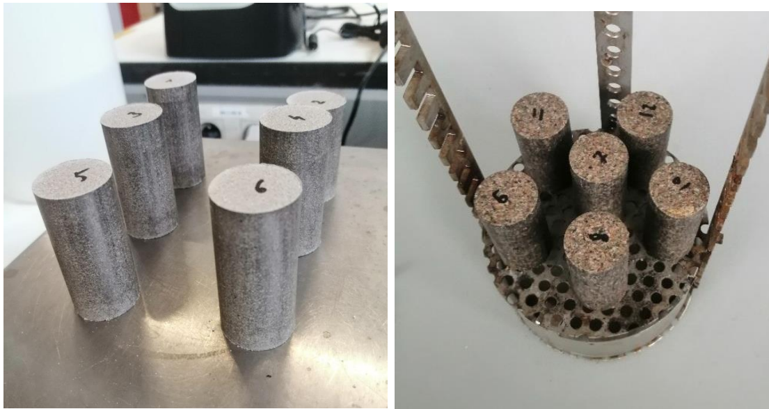
Figure 5-1. Carbonated cylinders made by hydraulic compaction of the RCF (left), RCA (right).
