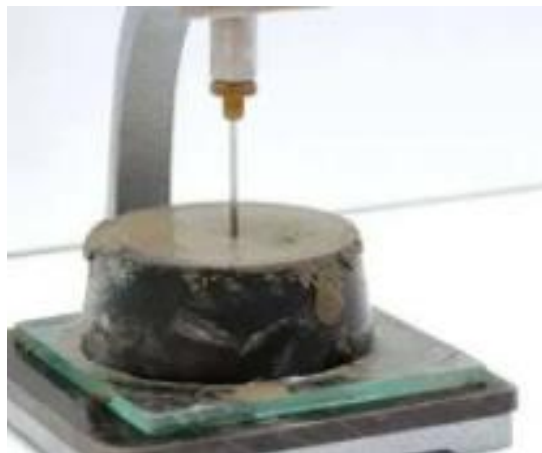
Figure 2-9 Cement Mortar Setting time test
