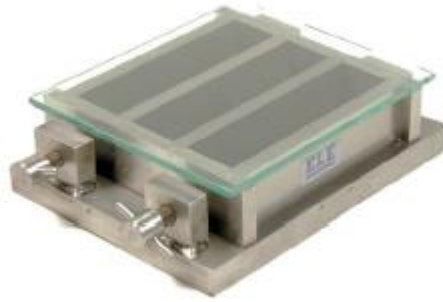
Figure 2-6 4x4x16 cm Cement Mortar Mold
