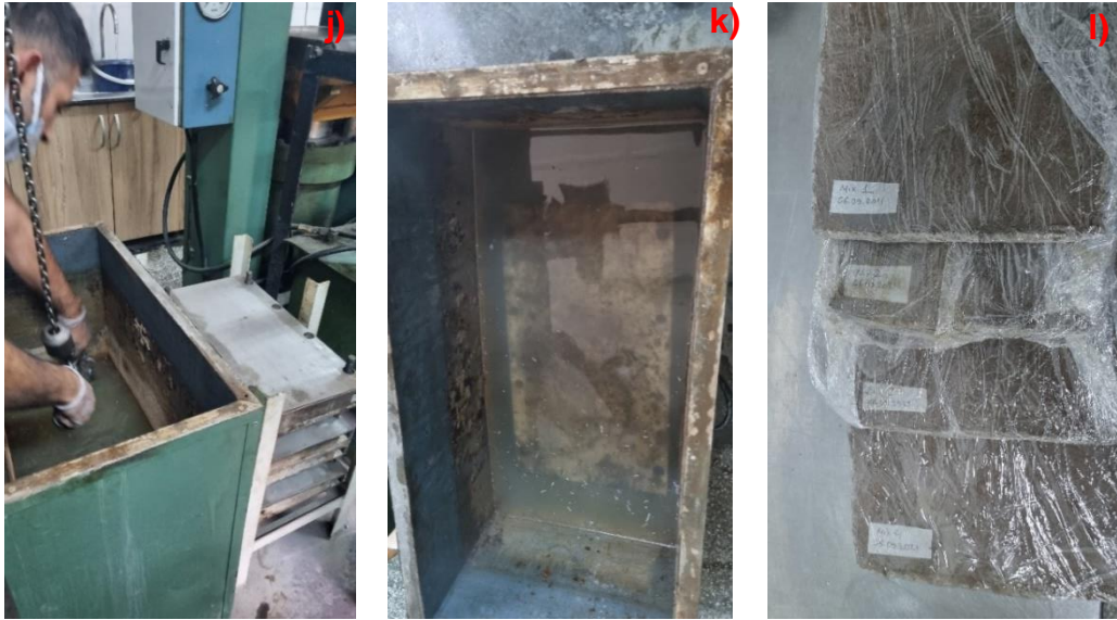
Figure 4-15 g) Press machine and pre-mold h) specimen before pressing i) specimen after pressing j) water curing at 85 °C k) cure pool l) specimen
