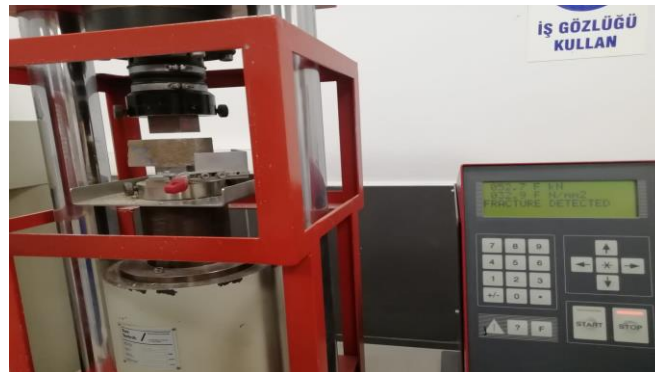
Figure 2-7 Cement Mortar Compressive Strength Test
