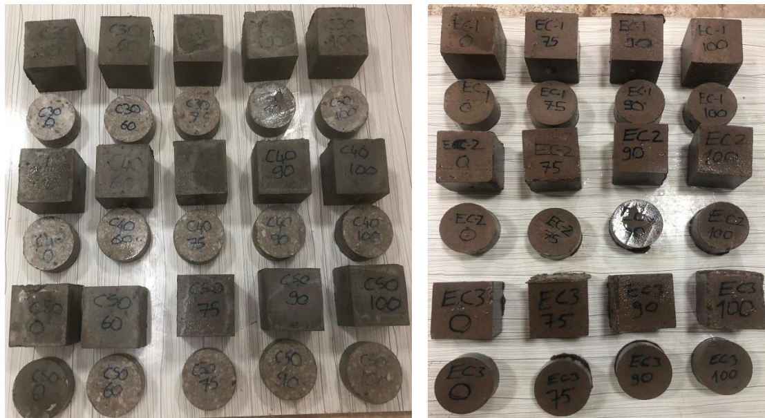
a) Cube and cylinder specimens produced with Portland cement
