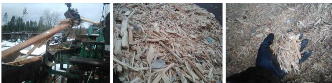
Figure 7-5. At left sorting and pre-crushing; on center and right, sort of Pin chips obtained for defibrating.
