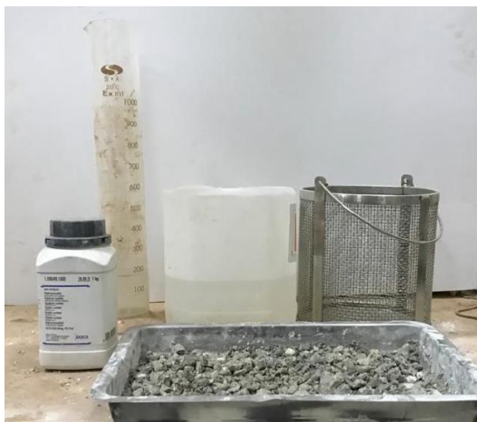
Figure 3-4 Sulphate soundness test equipment photo
