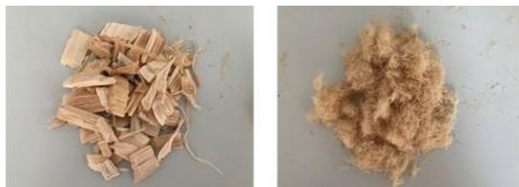
Figure 7-3. At left standard soft wood pin chips; at right wood fiber obtained from standard raw material.
