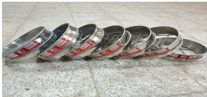
Figure 3-2 Sieves used for aggregate gradation.
