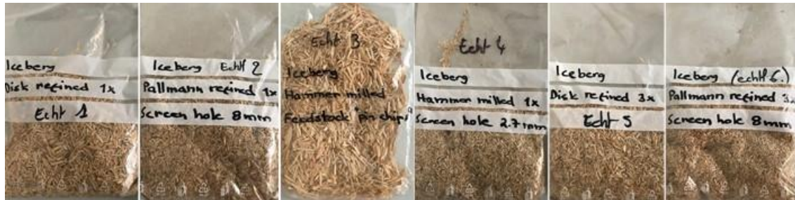
Figure 7-2 The first six kind of shredded C&D wood waste sample send from VTT.
