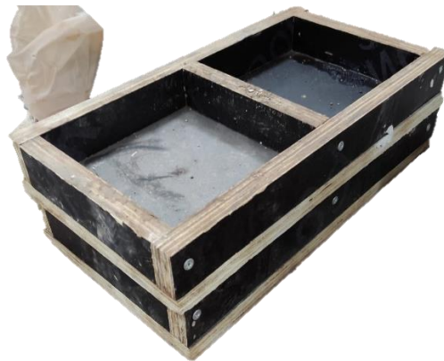
Figure 4-3 Image of the used molds for production of samples
