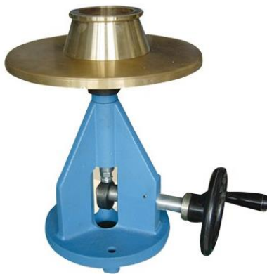
Figure 2-10 Cement Flow table test
