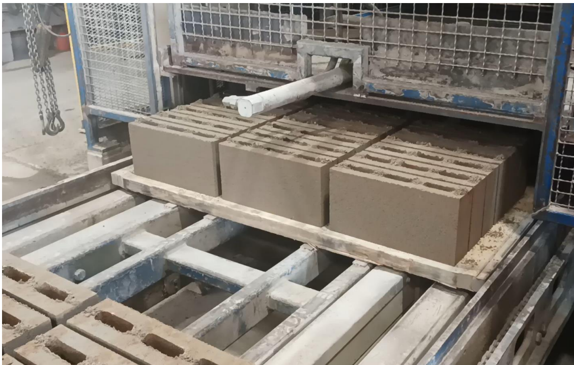
Figure 55. Produced blocks right after vibration pressing.
