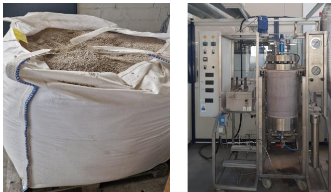
Figure 35. (a) 1m 3 of SC2 from GBN (b) 30 L reactor for Hydrothermal process
