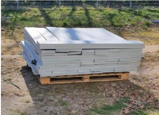
Figure 7. Collection of reusable ceiling plates (photographed by Frank Rens and Bente Kamp, GBN)
