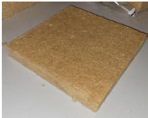
Figure 61. Insulation panel sample obtained from wooden demolition waste
