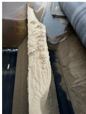
Figure 26. Accumulation of material on the splitter of the ADR
