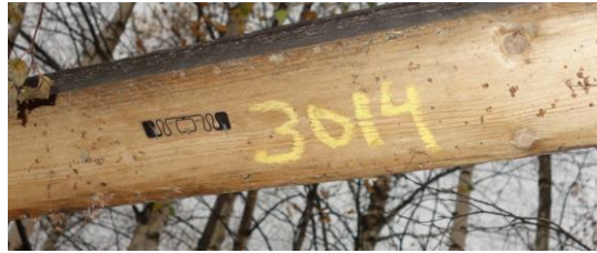
Figure 62. RFID tag attached to wooden construction part.
