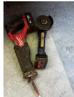
Figure 6. Hand tools used for pre-demolition
