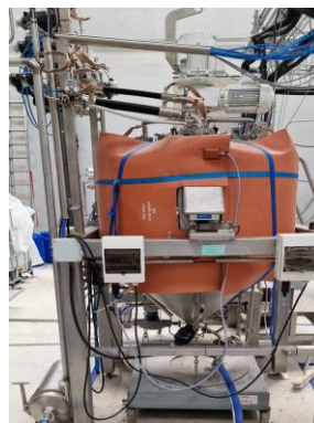
Figure 37. Silica aerogel synthesis reactor
