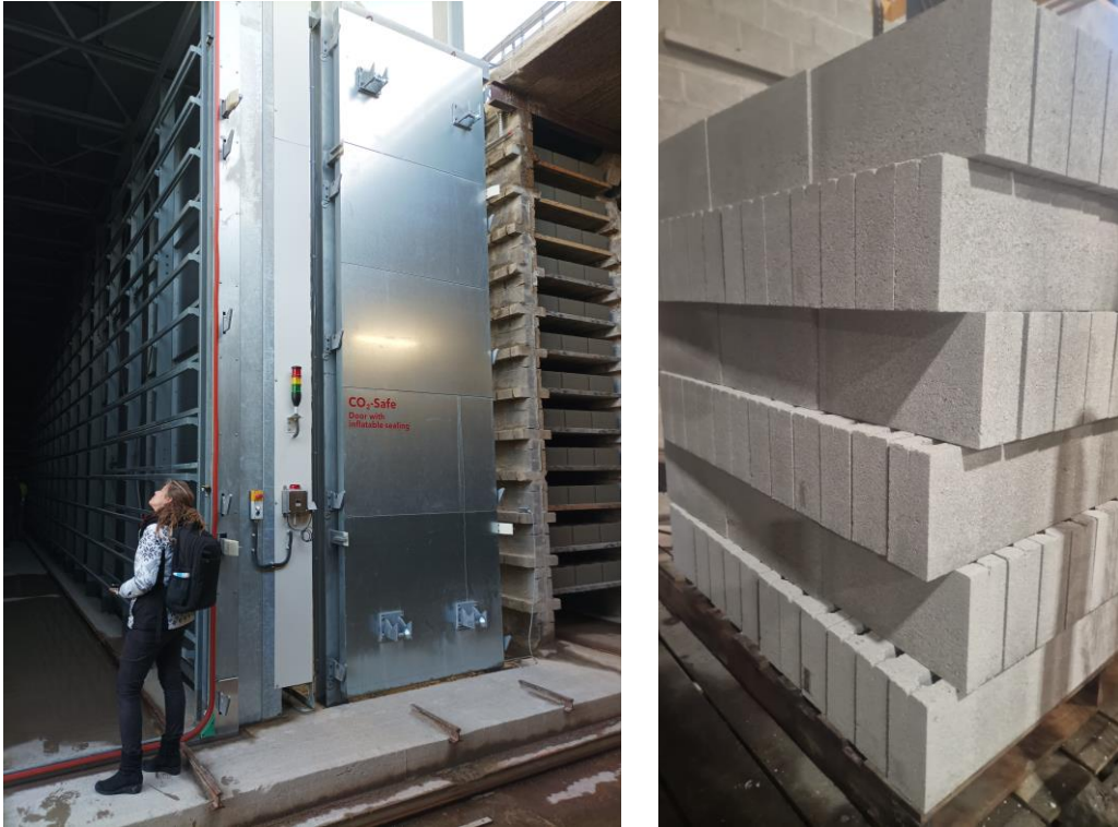
Figure 56. Carbonation chamber (left) and carbonated blocks (right).
