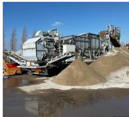
Figure 27. Fines produced with the ADR
