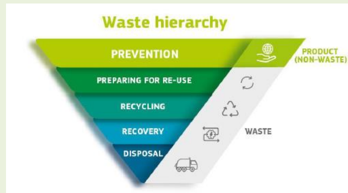
Figure 10 The waste hierarchy according to Waste Framework Directive. (ref. JRC EU Level(s) 37 )
