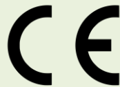
Figure 8 The CE marking indicates that a construction product is in conformity with its declared performance according to a harmonised European Product standard or according to a procedure set in a European Technical Assessment
